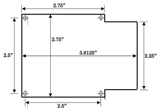
Figure 2-5. Manipulator base dimensions
