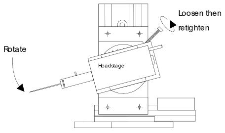
Figure 2-8. Adjusting the headstage angle
