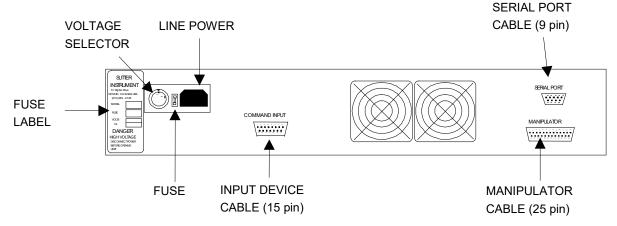
Figure 2-4. MP-285 controller rear connections
