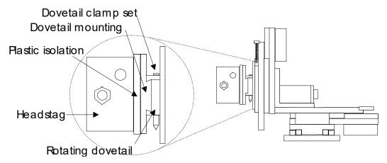
Figure 2-7. Mounting the headstage on the manipulator's Z-axis
