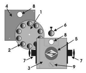
Figure 1-1. Lambda series 25mm filter wheel (without shutter).
