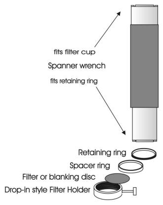
Figure 2-4. Filter holder components.
