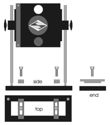
Figure 2-2. Filter wheel-mounting stand.
