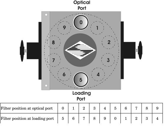
Figure 2-8. Filter ports (plug is removed from the loading port).
