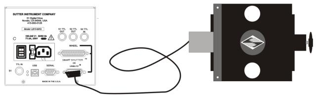
Figure 2-3. Filter wheel connection
