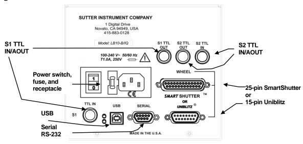
Filter wheel with optional SmartShutter or Uniblitz shutter (25- or 15-pin cable) configuration
