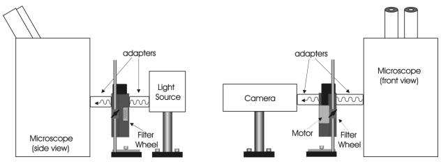
Figure 2-1. Schematic diagram of two possible experimental configurations.
