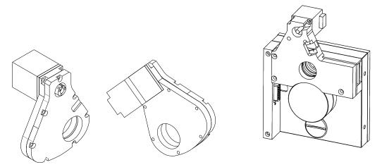
Figure 1-4. 25mm SmartShutter standalone and mounted on the housing of a 25mm filter wheel.
