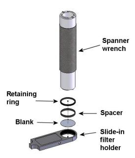
Figure 2-5. Changing filters in the Slide-In Filter Holder.
