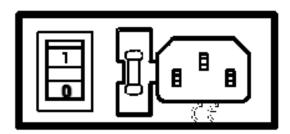
Figure 3-2. Switch, fuse, and power connection.
