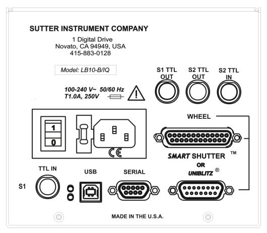
Figure 1-7 Rear panel electrical connections.
