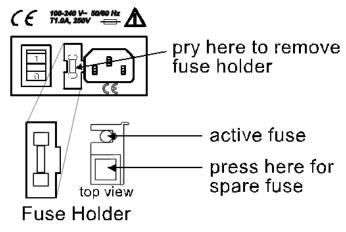
Figure C-1. Power entry module and fuse holder.
