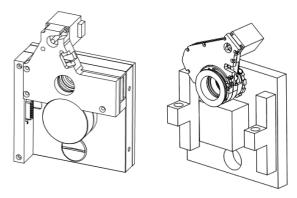
Figure 1-3. Lambda-series 25mm filter wheel housing with 25mm SmartShutter and 32mm filter wheel housing with 35mm SmartShutter.
