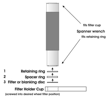
Figure 2-6. Removing the retaining ring.
