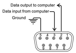
Figure 6-1. Serial port pin assignments.
