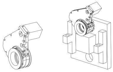
Figure 1-5. 35mm SmartShutter standalone and mounted on the housing of a 32mm filter wheel.
