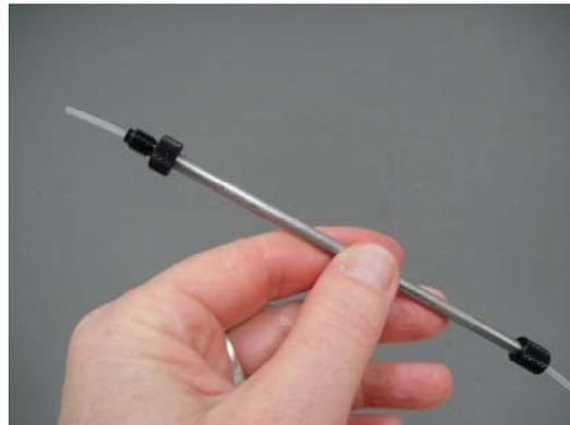
3. Remove the front connector of the pipette holder. Insert tubing from the back end through the front and make sure the black metal ends are screwed on tight.
