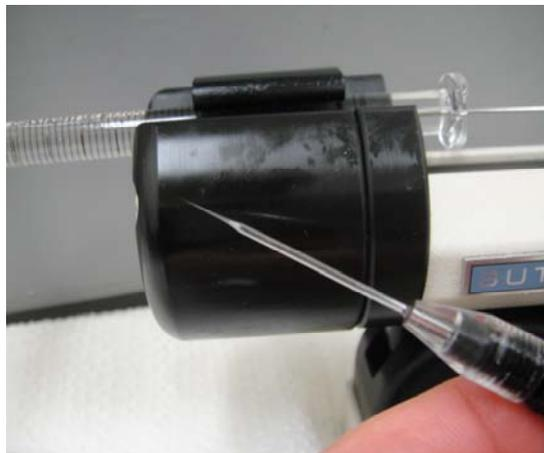
8. Turn the clear plastic tip of the pipette holder ½ turn to loosen the seal, allowing you to insert your pipette. Push the pipette all the way into the holder (the o-rings might offer some resistance) until it goes not further. The holder is designed to accept 1mm outer diameter glass. If you are using glass with a 1.2mm or 1.5mm OD, contact Sutter Instrument to purchase a custom holder to accept the size of your glass.
