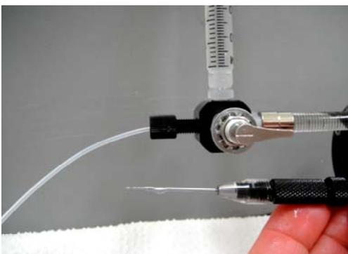
3. Replace the pipette and turn the selector back facing east. Then use the coarse dial on the injector or the 3cc syringe to fill the pipette.
