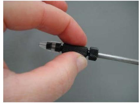
4. Slide the plastic ferrule onto the tubing as shown above, press the ferrule and tubing flush to the male connector, then replace the front female connector and screw it on so it is very firmly seated.
