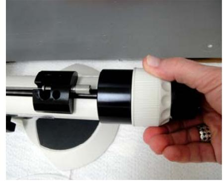
1. If the volume in the Hamilton syringe gets low, first remove the pipette and reattach the 3cc filling syringe. Then turn the selector east. Use the coarse dial on the Injector (counter clock-wise) to draw oil/water into the Hamilton syringe.
