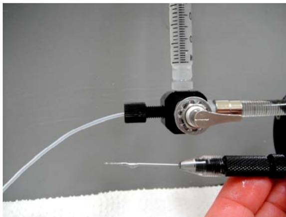
9. With the selector facing east, use either the 3cc syringe or the Hamilton syringe (by turning the coarse dial on the XenoWorks injector) to fill the pipette and advance the oil/water all the way to the tip.
