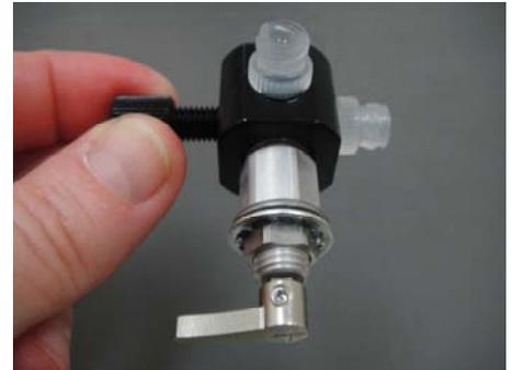
5. Insert tubing through rear connector and install the ferrule. **First** attach the 3-way connector to the Hamilton syringe and **then** attach rear connector to the three-way valve.
