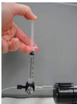
2. Turn the selector north and use the 3cc syringe to re-refill the tubing and advance the oil/water to the tip of the pipette holder
