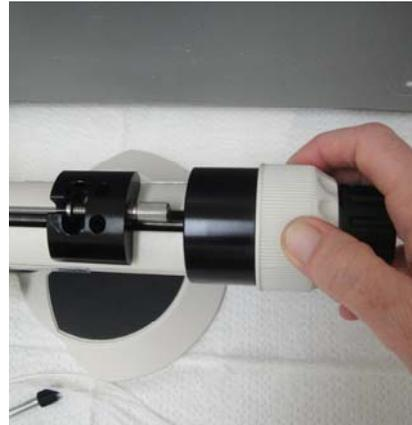
6. Fill a 3cc syringe with oil or water and make sure there are no air bubbles. Screw it onto the top port of the 3-way valve and position the selector east. Then turn the coarse dial of the injector clockwise six complete turns to advance the plunger and introduce oil/water into the 3-way valve.
