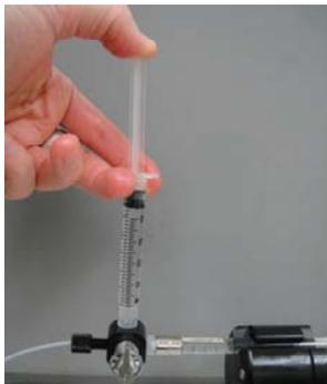
7. Tighten the clear plastic tip of the pipette holder (without a pipette installed) and use the 3cc syringe to advance oil/water into the tubing and to the tip of the pipette holder. Advance the oil/water until all air bubbles are flushed out.
