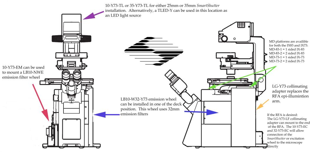
Filter wheel and SmartShutter adapter guide for the Olympus IX3 microscope
