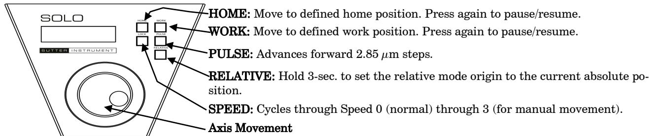
**Setting Home/Work Pos. & Relative Mode Origin Pos.:** To set position, hold down HOME, WORK, & RELATIVE buttons for 3 seconds until beep sounds.
