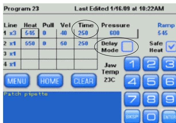
Figure 16. Time mode of air-cooling.
