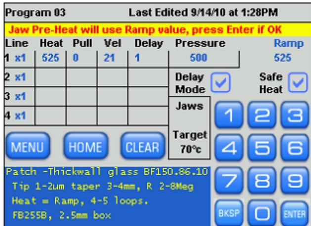
A caution is displayed indicating that the filament will light up and pre-heat. This yellow message bar is displayed when powering up and entering a Pre-Heat program; when waking from sleep; and when going from a non-Pre-Heat program into a Pre-Heat program.
