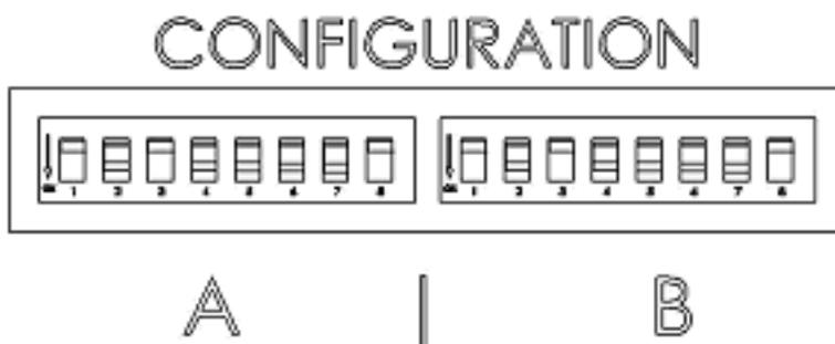
Figure 2-5. Configuration switches (rear of MPC-200 controller).
