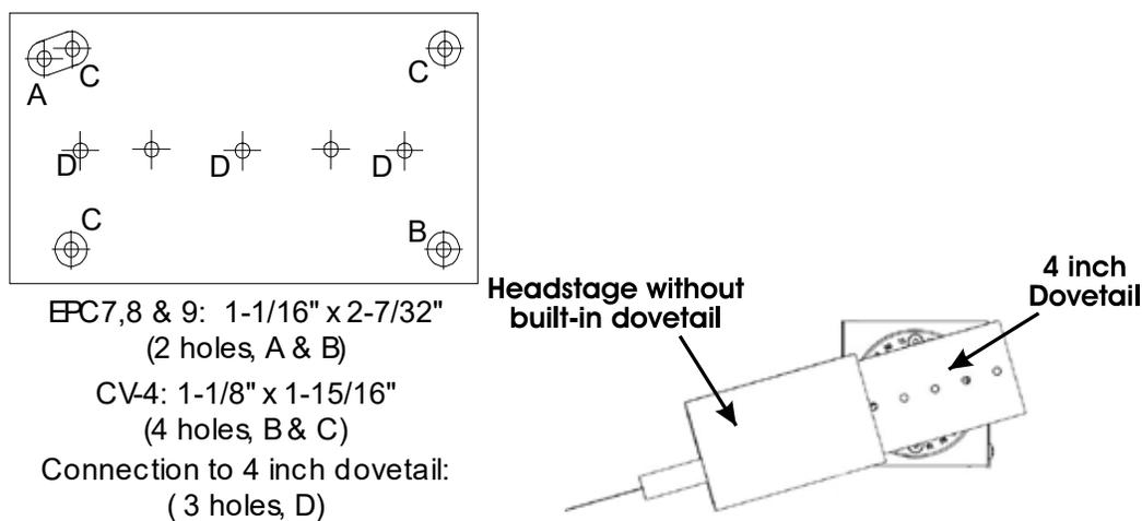
Figure 3-5. Using a dovetail for headstage mounting.
