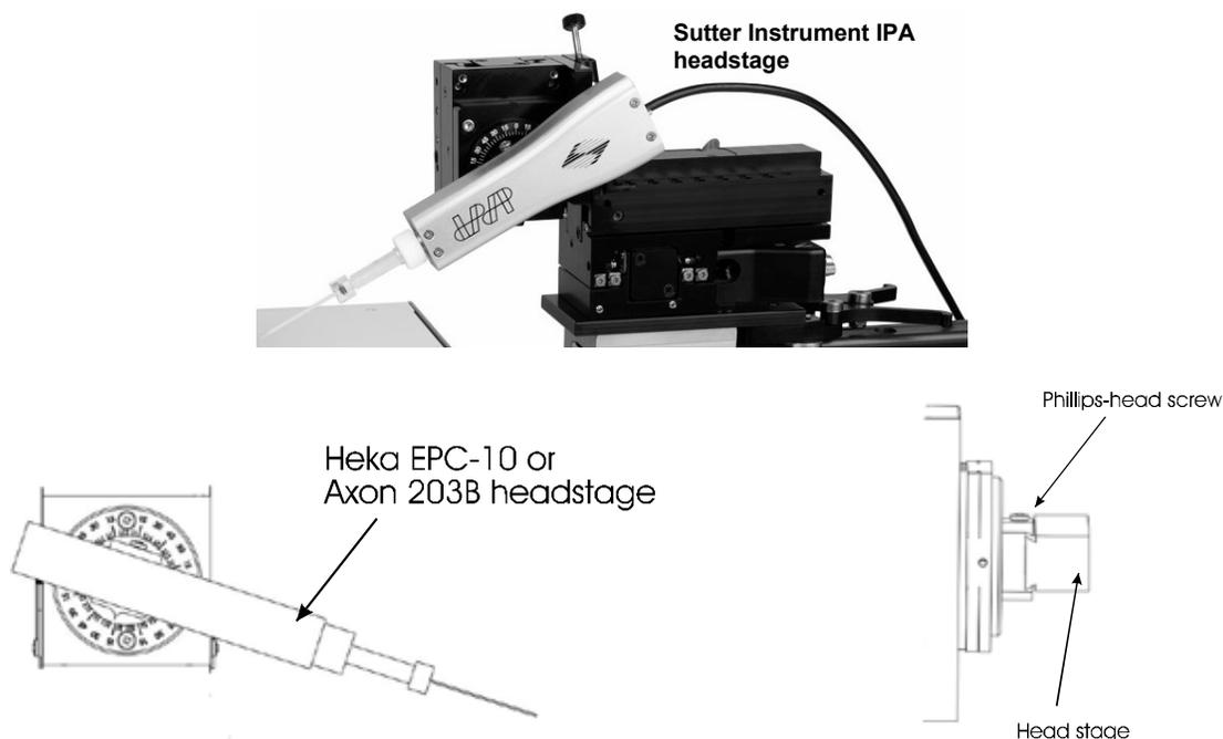
Figure 3-4. Headstage mounting.
