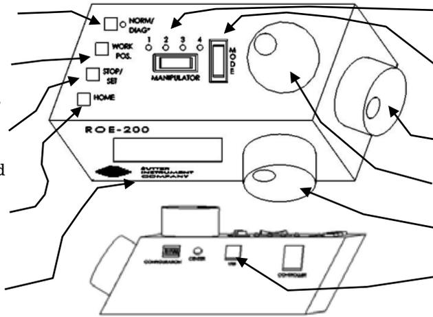
**MANIPULATOR:** Selects Manipulator 1 through 4 (as connected).
