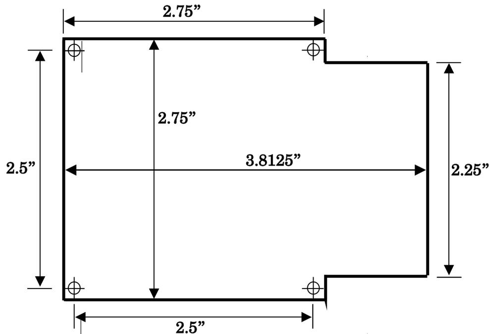
Figure 2-5. Manipulator base dimensions
