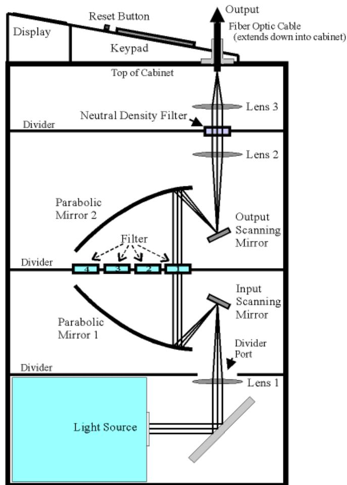
Figure 1-1. Lambda DG-4/5 optical pathway.
