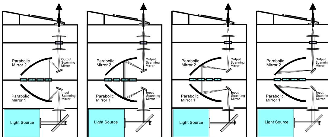
Figure 3-5. DG-4/5 output attenuation.
