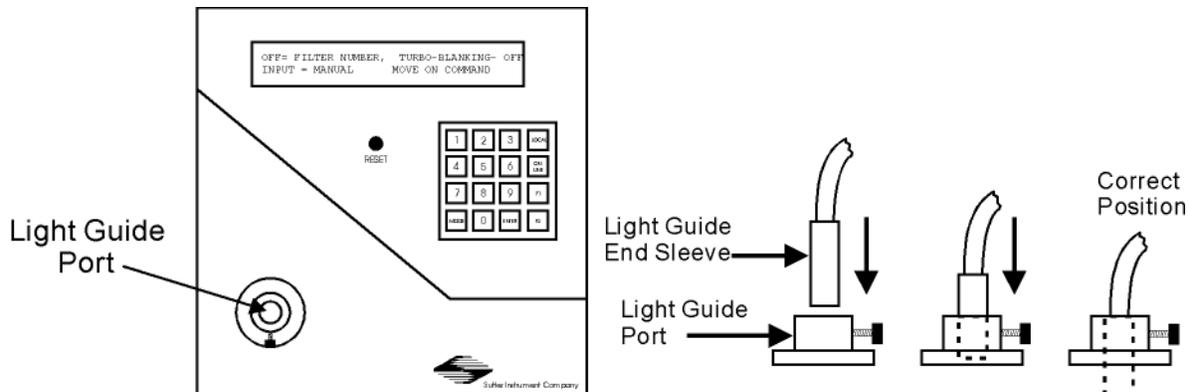
Figure 2-3. Liquid light guide installation.
