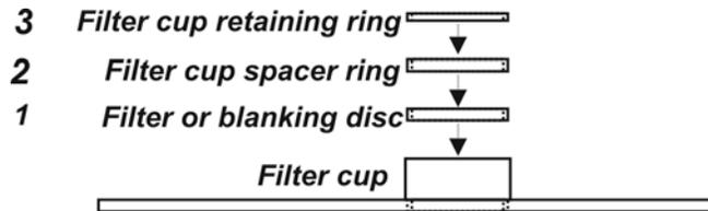
Figure 2-6. Filter holder assembly with blanking disc.
