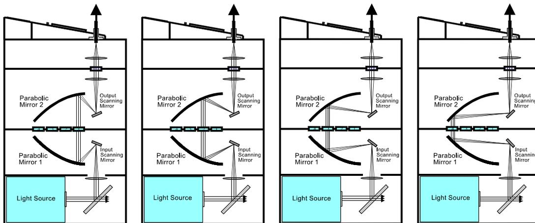
Figure 3-4. Optical pathway based on filter position.
