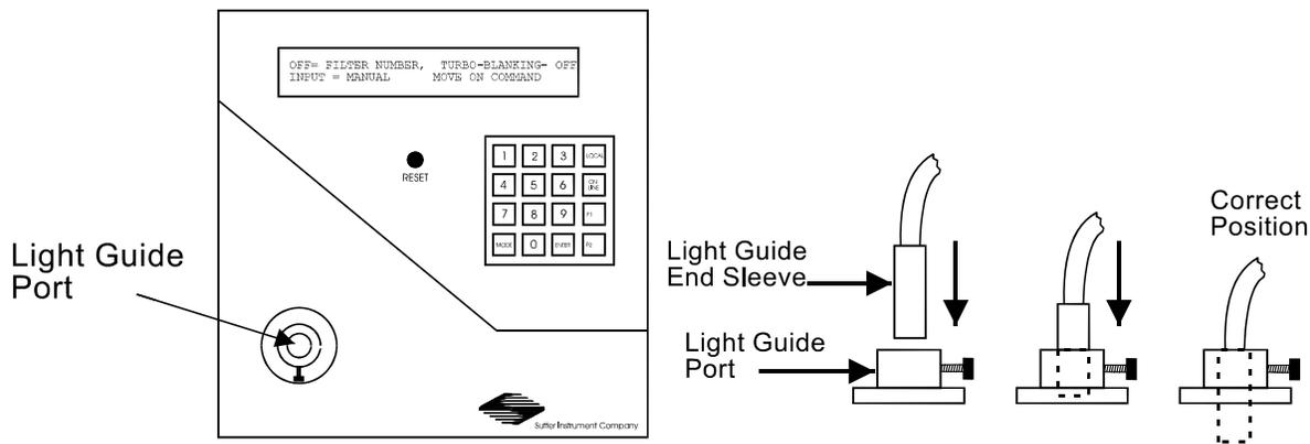
Figure 2-3. Liquid light guide installation.
