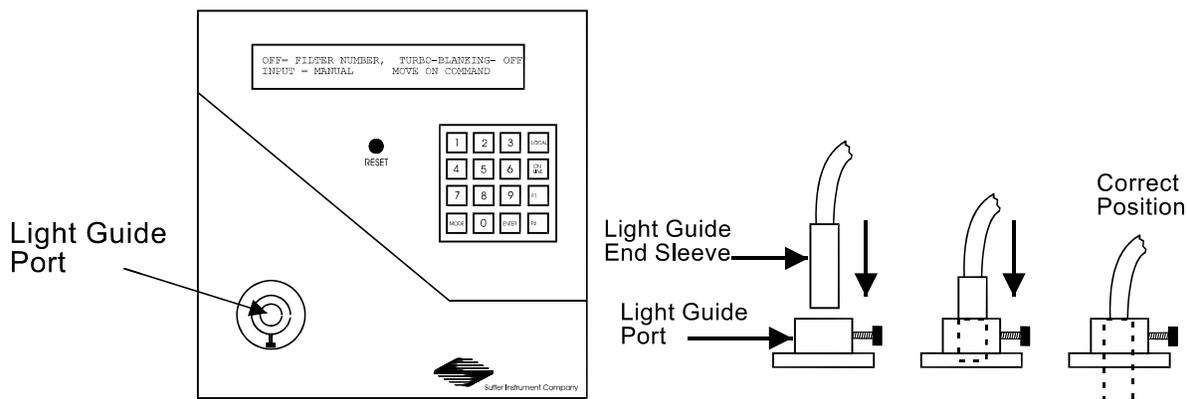
Figure 2-1. Light guide installation.
