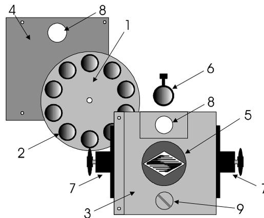
Figure 7-1. Lambda 10-C Filter Wheel (without shutter)
