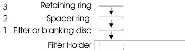
Figure 7-6. Assembly order of filter holder parts
