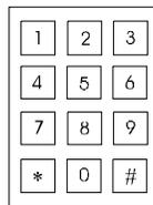
There are 12 keys on the Lambda 10-C keypad. The numerical keys 0 to 9 and two function keys (\* and #). Keys are read while depressed but the appropriate action will occur only when the key is released. If a key is pressed while a move is in progress but released after the move is over, the key will read normally. Keys pressed and released while a move is in progress are ignored..
