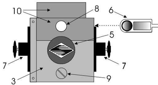
Figure 7-2. Lambda 10-C filter wheel housing (with shutter)
