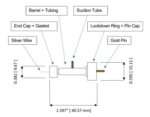
Figure E-0-1. Electrode Holder Figure dimensions are in "inches [mm]".
