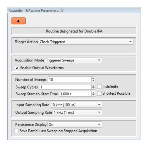
Figure 4-54. Acquisition & Routine Parameters
