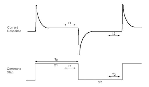
Figure 0-1. MT Command Pulse & Response
