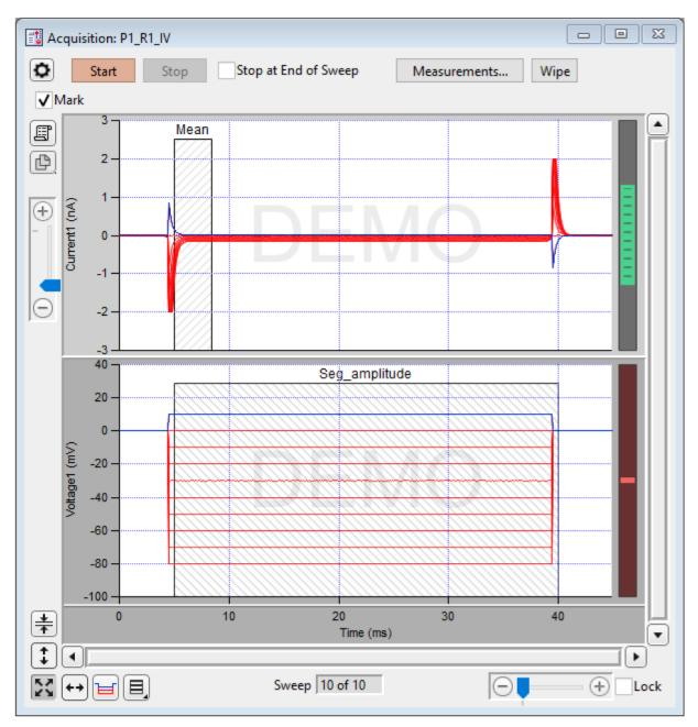
Figure 4-3 Acquisition: Routine Scope Window
