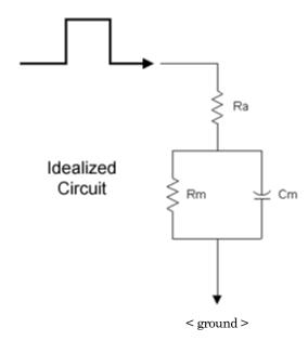
Figure 0-2. Idealized Membrane Circuit
