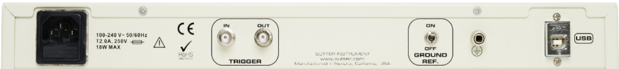
Figure 3-2. Rear of Dendrite Cabinet
