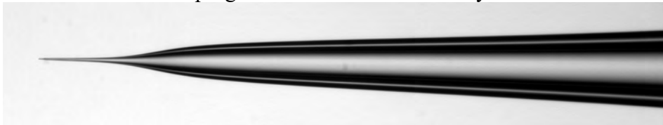
Image B (40x mag.) 1.0 x 0.5 thick-walled glass (BF100-50-10) ~0.5µm Tip, w/ a shorter taper than that shown above. Three-line program with a reduced velocity on Line 3
