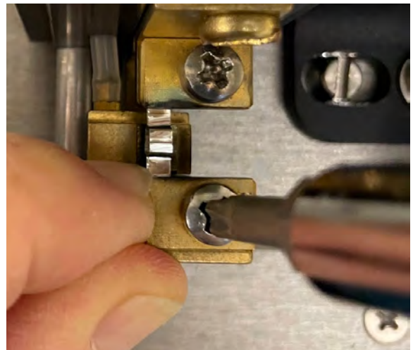
Firmly hold the inside left corner of clamp before tightening the screw to prevent clamp from twisting and distorting the filament.
