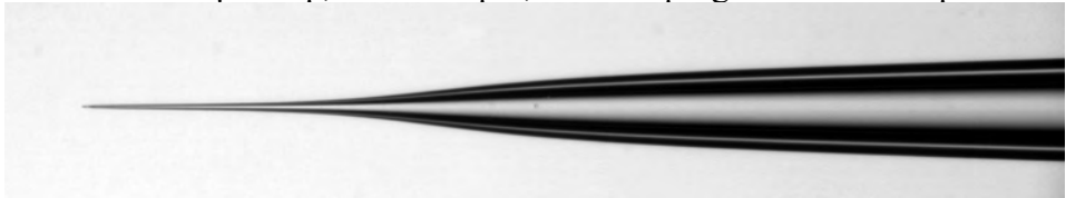
Image A (40x mag.) 1.0 x 0.5 thick-walled glass (BF100-50-10) ~0.5µm Tip, 4-5mm taper, one line program with 3 loops
