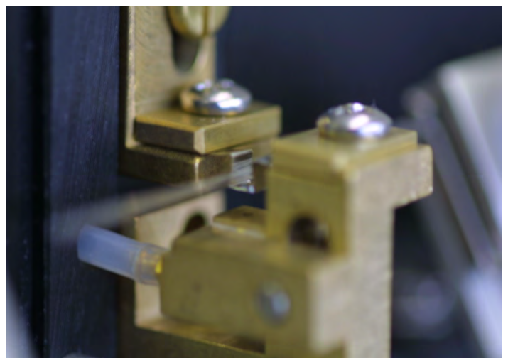
Good - Glass sitting low and 0.5 to 1mm above the base of a Trough Filament
