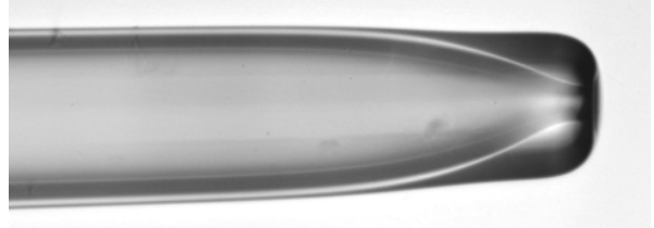
Medium Holding Pipette (400x mag.) Scored with cut using the Ceramic Tile 50 \mu m OD x 20 \mu m ID, medium polish
