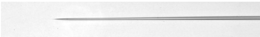
0.7 - 0.9 \mu m tip, 5 - 7mm taper (400x)
