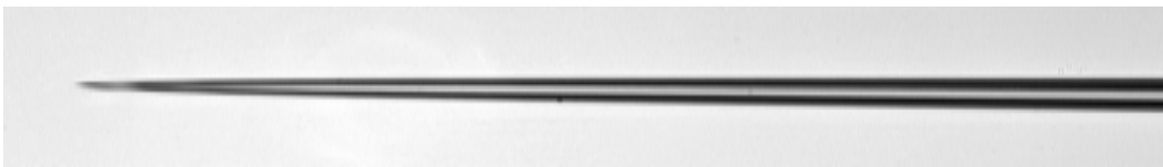
0.6 - 0.9 \mu m tip, 6 - 8mm taper (400x)
