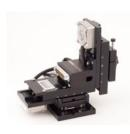
The MP-285 is suitable for patch clamp experiments, extracellular recording, microinjection, intra-cellular recording and precision robotic positioning applications. Max speed 5 mm/sec.
