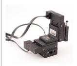
The MP225 features linear bearings and a modularized, compact design easily adaptable to your setup. 25 mm of travel on all three axes with max speed of 3 mm/sec.
