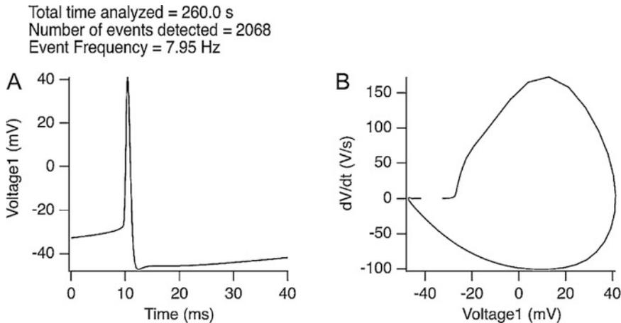
**Fig. 8** Graphical output of the SutterPatch Action Potential Analysis Module applied to a recording of spontaneous activity in a brain slice. **(a)** Average action potential waveform across all detected events. **(b)** Phase-plane plot of the averaged action potentials. Above the plots, basic statistics of the analyzed dataset are put out. In addition to the layout, the numerical results for each action potential are compiled and displayed as a table (not shown)
