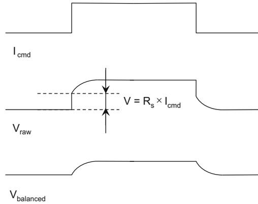
**Fig. 5** Bridge balance compensation. A command step applied in current clamp ( $I_{cmd}$ ) elicits a voltage drop across the pipette resistance, superimposed by the voltage response from the preparation ( $V_{raw}$ ). Bridge balance compensation eliminates the Ohmic portion and returns the isolated voltage response from the preparation ( $V_{balanced}$ )
