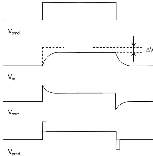
**Fig. 4** Series resistance correction and prediction. The command step  $V_{cmd}$  is both reduced in amplitude and slowed down by the series Resistance, which results in the membrane potential  $V_m$ . Series resistance correction ( $V_{corr}$ ) and prediction ( $V_{pred}$ ) mitigate this effect, depending on the percentage applied and square up  $V_m$  (not shown)
