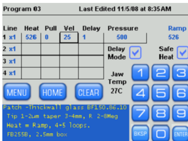
Figure 4-18. Examining the contents of a program using the Program Edit screen.
