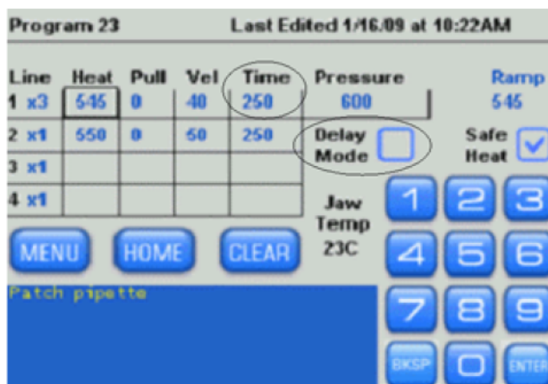
Figure 2-16. Time mode of air-cooling.
