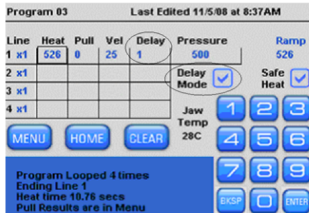
Figure 2-17. Delay mode of air-cooling.
