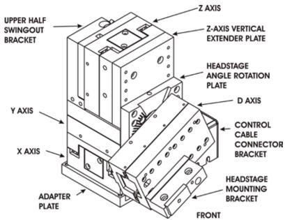
Figure 2-1. Angled side view of QUAD/M showing mounting adapter plate.
