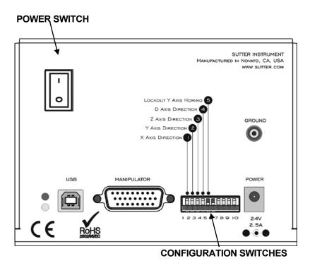
Figure 2-4. Rear panel of QUAD ROE/Controller cabinet.
