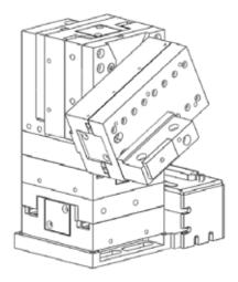
$\label{eq:Figure 6-1.Default Rotator/D-Axis mechanism} Figure \ \ 6-1. \ Default \ Rotator/D-Axis mechanism mounting position.$
