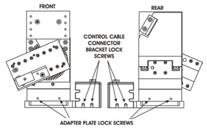
Figure 2-2. Locations of Mounting Bracket and Connector Bracket lock screws.
