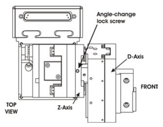
Figure 3-12. Top view of QUAD/M showing lock screw for headstage/pipette angle change.
