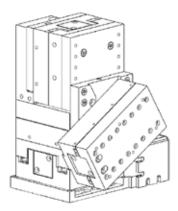
$\begin{array}{cccc} Figure & \hbox{6-5. The QUAD/M showing the Rotator and D-} \\ Axis at a lower position on the Z-Axis. \end{array}$
