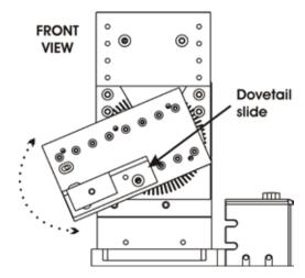
Figure 3-2. Front view of QUAD/M showing D-axis rotation.
