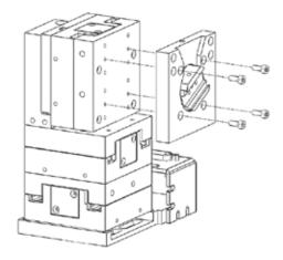
Figure 6-2. Removing the Rotator Plate from the Z-Axis Plate.
