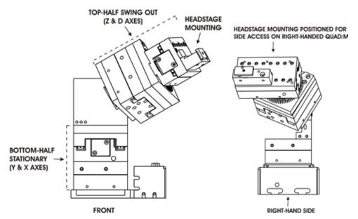
Figure 3-13. Swinging out the top half of the QUAD/M for side access to headstage mount.
