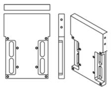
Figure 2-3. QUAD/M Adapter Plate.
