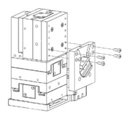
Figure 6-4. Installing the Rotator to the lower position on the Vertical Extender Adapter.
