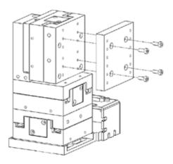
Figure 6-3. Installing the Vertical Extender Plate to the Z-Axis Plate.
