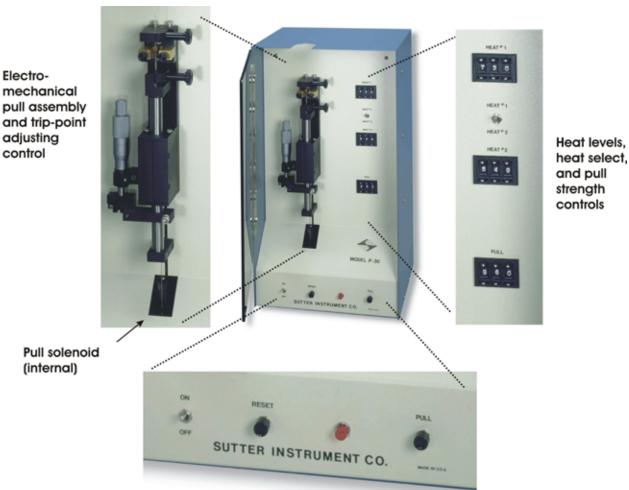
Power, reset, and pull controls, and power indicator Figure 1-1. Front panel components.
