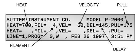
Figure 3-4. LCD Display (program parameters)
