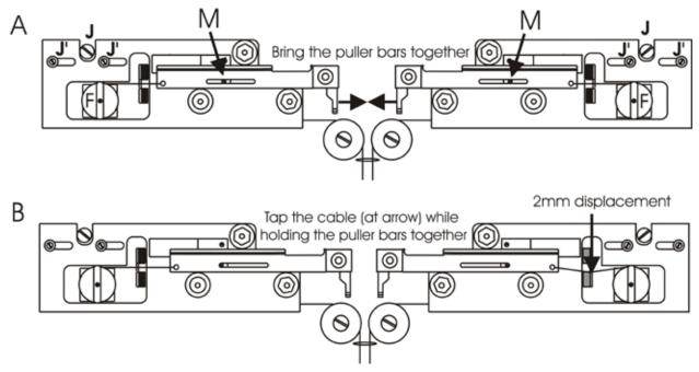
Figure 5-6. Pulley adjustment
