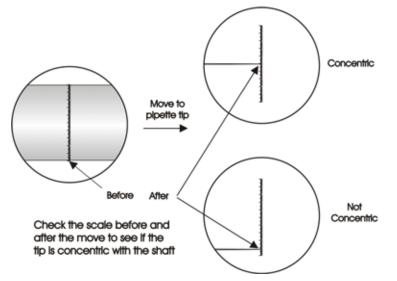
Figure 4-3. Field of view when checking the concentricity
