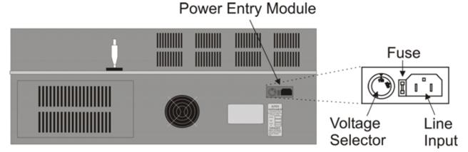
Figure 6-1. Power entry module
