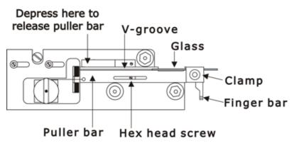
Figure 3-1. Left Puller Bar
