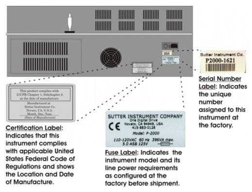
Figure 1-1. Information labels on the back of the P-2000 cabinet.
