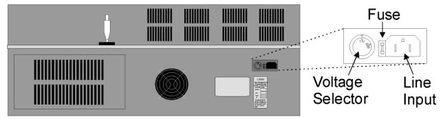
Figure 2-2. P-2000 Cabinet (rear view)
