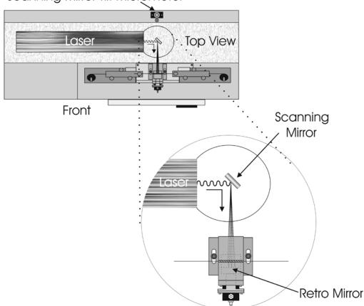
Scanning Mirror Tilt Micrometer
