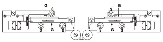
Figure 5-1. V-groove bearings and pull bars.
