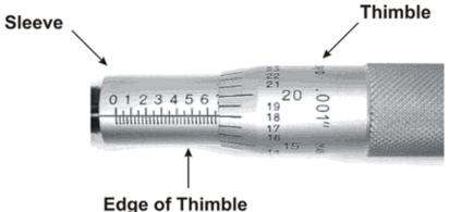
Figure 5-3. Micrometer scale
