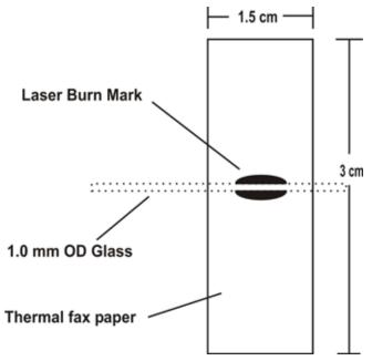
Figure 5-4. Scanning mirror adjustment using thermal paper.
