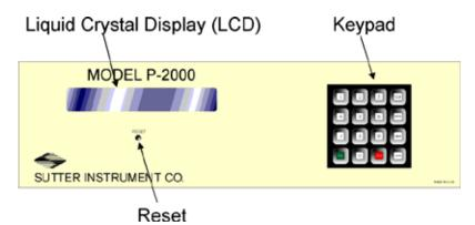
Figure 3-2. P-2000 Front Panel
