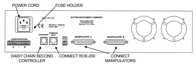
Figure 2-1. Rear of MPC-200 controller cabinet.
