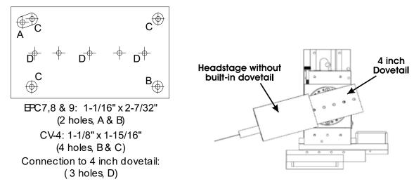
Figure 3-4. Using a dovetail for headstage mounting.
