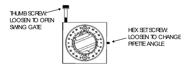
Figure 3-2. Locations of screws used to open swing gate and changing pipette angle.
