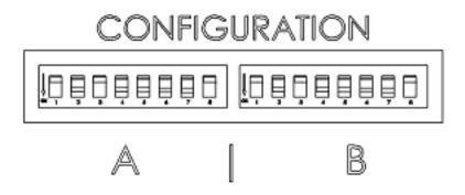
Figure 2-4. Configuration switches on rear of MPC-200 controller cabinet.
