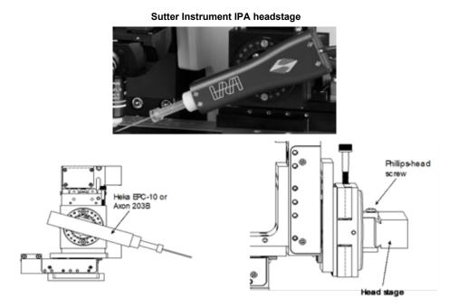
Figure 3-3. Headstage mounting.
