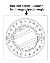
Figure 3-3. Location of screw to loosen for changing pipette angle.
