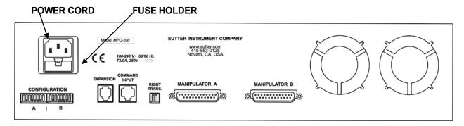
Figure 4-1. MPC-200 Controller cabinet (rear view) showing power connection and fuse.
