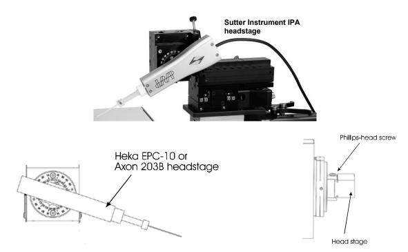
Figure 3-4. Headstage mounting.
