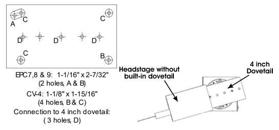
Figure 3-5. Using a dovetail for headstage mounting.
