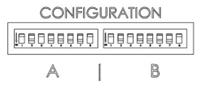
Figure 2-5. Configuration switches (rear of MPC-200 controller).
