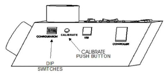
Figure 1. Location of the CALIBRATE button on the ROE-200.
