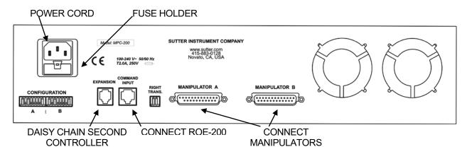
Figure 2-1. Rear of MPC-200 controller cabinet.
