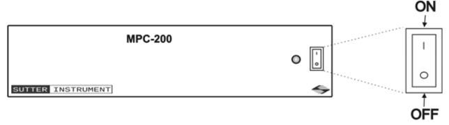
Figure 4-2. Power switch (front panel).
