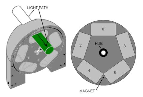
Figure 1-1 Anatomy of the Lambda VF-5 filter wheel.
