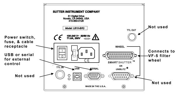
Figure 1-3. Electrical connections.
