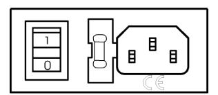
Figure 3-2. Switch, fuse, and power connection.
