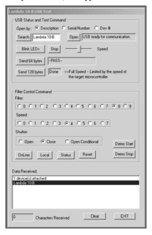
Figure 7-9 -- USBTest main screen.
