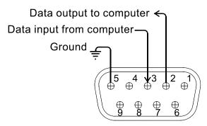
Figure 6-1. Serial port pin assignments.
