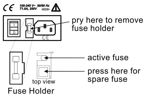
Figure 8-1. Power entry module and fuse holder.
