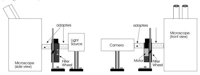
Figure 2-1. Schematic diagram of two possible experimental configurations.
