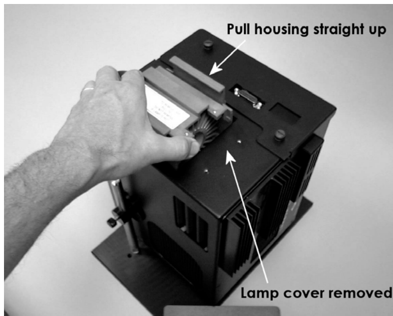
Figure 3-2. Removing the bulb assembly from the Lambda-LS.
