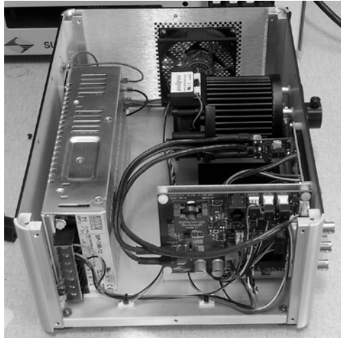
Figure 2-1. Lambda HPX-series left-side panel removed for access to configuration DIP switches.
