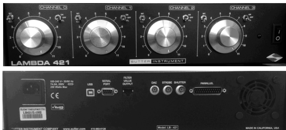
Figure 3-1. Locations of individual indicators, controls, and connectors on the Lambda 421 controller.
