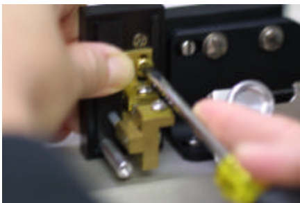
STEP 1. Loosen top brass screw then...
