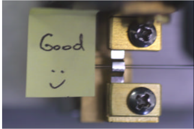
Box filament centered over the air jet and is 1.0mm in from the left edge of the brass jaws. The filament is positioned so the glass runs through the center of the filament. This is GOOD!
