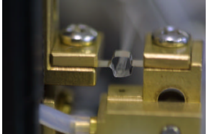
GOOD... jaws even, glass centered, air jet 3mm below the filament.
