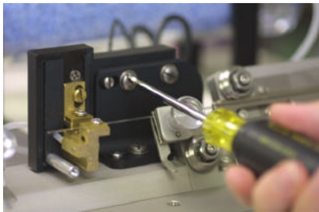
Loosen the locking screw
